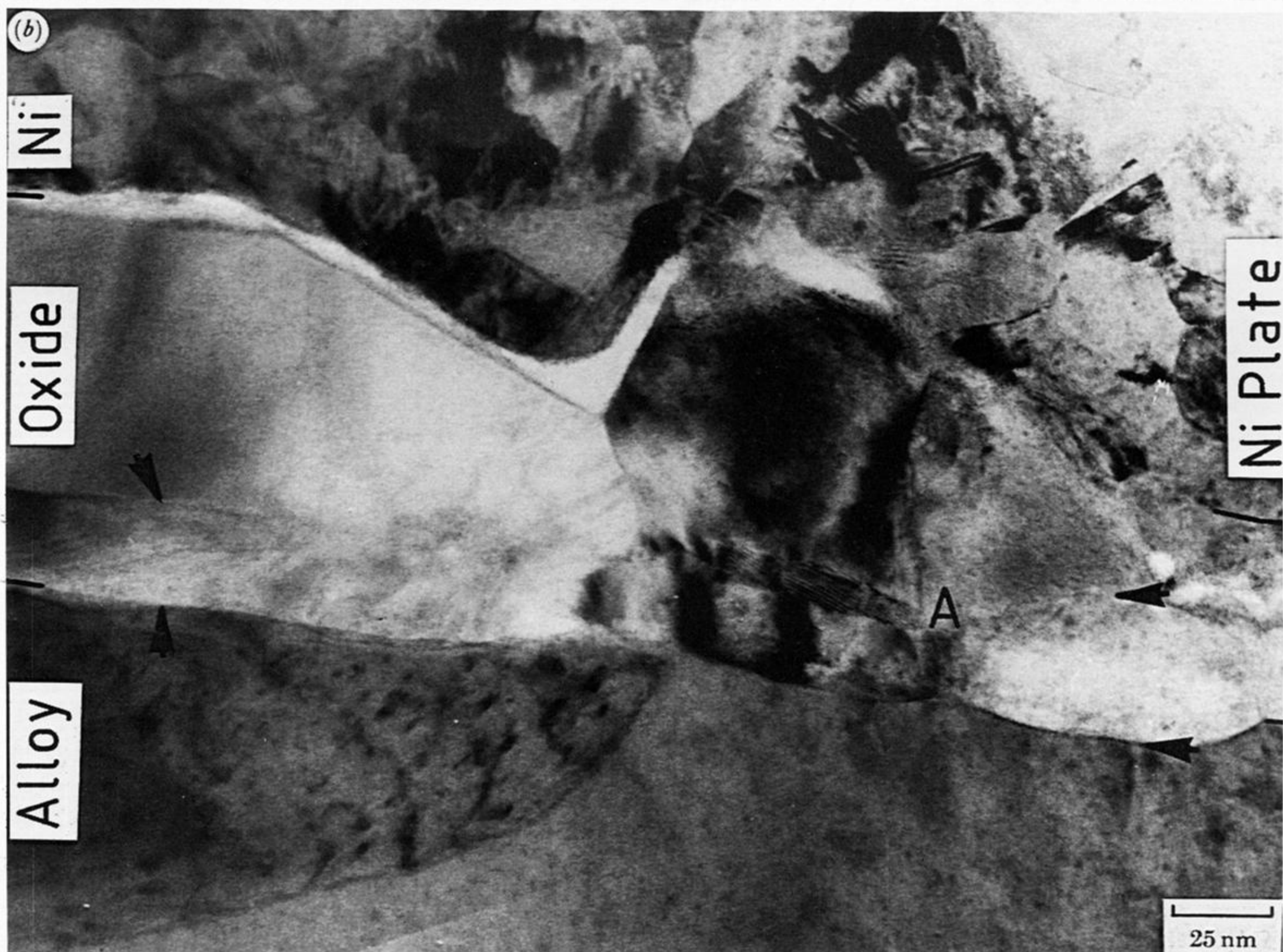
FIGURE 9. Fe-20Cr-34Ni oxidized for 6 h in air at 600 °C. 'Edge-on' bright-field micrographs showing (a) a low magnification image of a thin oxide layer ( M_2O_3 ) sandwiched between the alloy and nickel plate, as arrowed (note the relatively fine alloy grains immediately beneath the scale); (b) a higher magnification image of the two-layered oxide morphology where the thinner and innermost layer is delineated by arrows (note the cusped morphology of the scale at the alloy-oxide and oxide-nickel plate interfaces).
