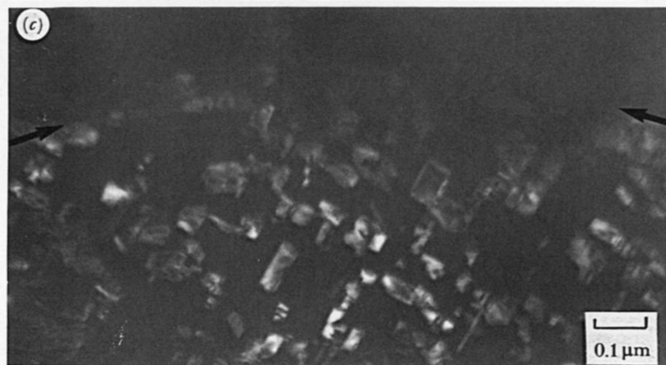
FIGURE 20. Fe-20Cr-20Ni oxidized in 1% CO-CO 2 for 1000 h at 600 °C. (a) Bright-field micrograph of the alloy scale interface showing equiaxed oxide grains which again have a cusped morphology. The inset shows a (\bar{1}2\bar{1}6)_{\text{Cr}_2\text{O}_3} diffraction pattern. (b) Bright-field and (c) dark-field micrograph (imaged with a (200) carbide reflection showing \text{M}_{23}\text{C}_6 precipitates in the alloy. The interface between the recrystallized and bulk alloy (see figure 19) is arrowed in (b) and (c). It is apparent that carbide precipitation has not occurred in the recrystallized region of the alloy. (d) (310)_{\gamma} // (310)_{\text{M}_{23}\text{C}_6} diffraction pattern.
